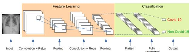
Fig. 3: Structure of proposed DLA CNN-based
